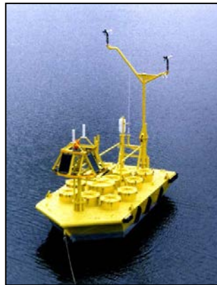
Figure 3-8b 6-meter Boat-shaped Hull Buoy
