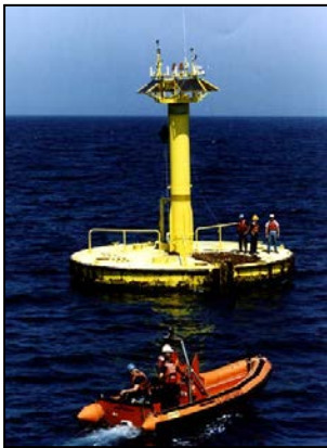
Figure 3-8a 10-meter Discus-shaped Hull Buoy
