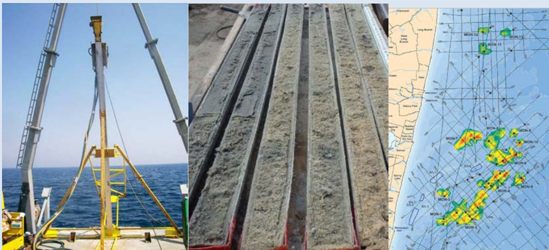
Vibracore Sampling, Split Vibracore, and Significant Sand Resources off Monmouth County, NJ
