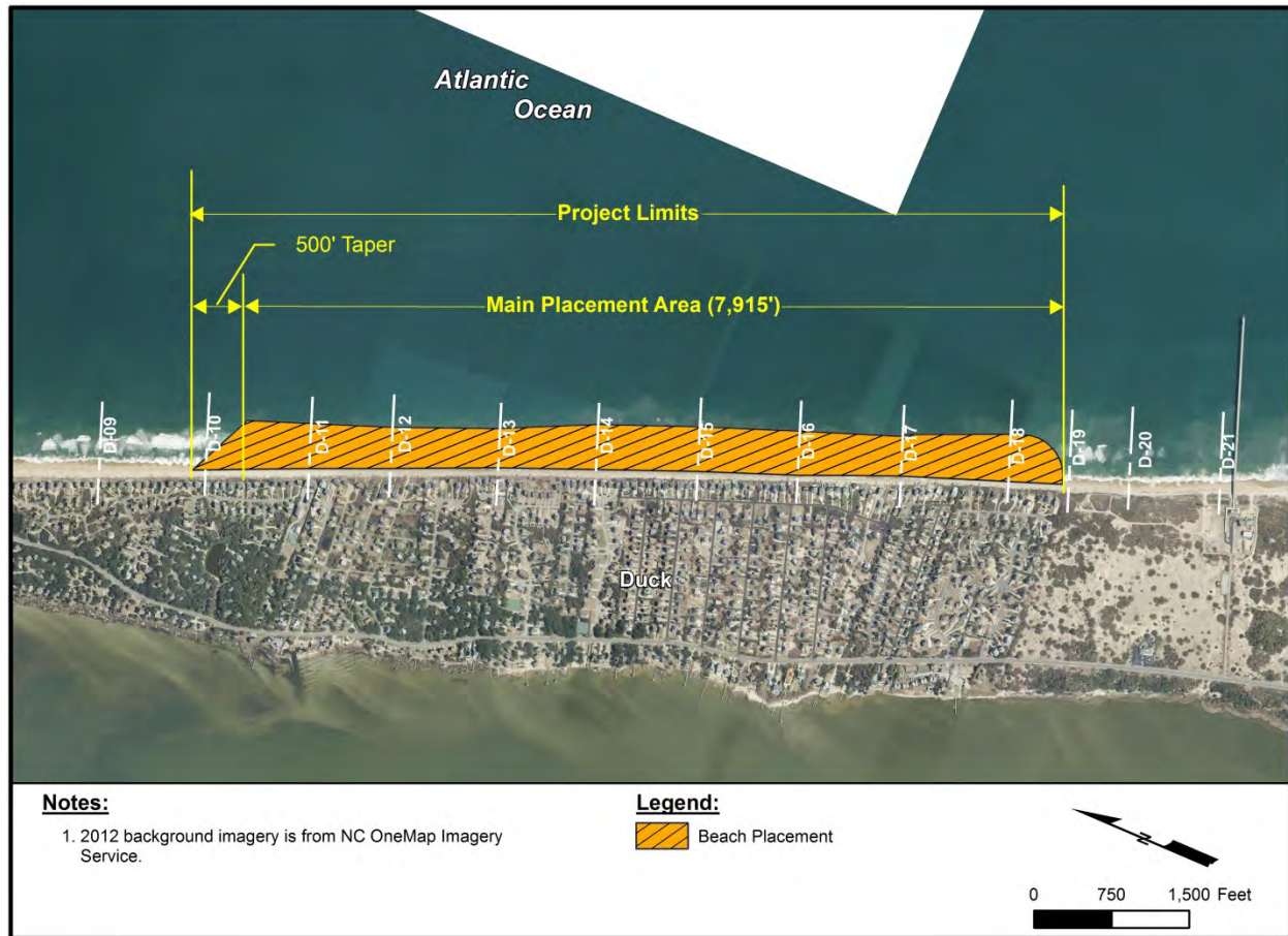
Figure 2. Project design for the Town of Duck, including the project limits, main placement area and tapers.
